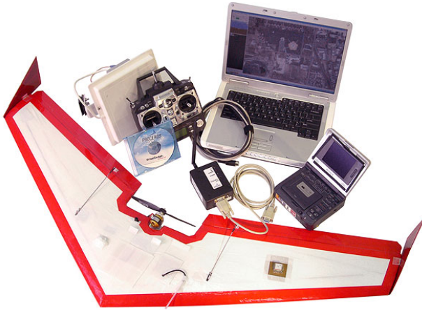
Fig. 8 Procerus Unicorn UAV test aircraft with accessories
