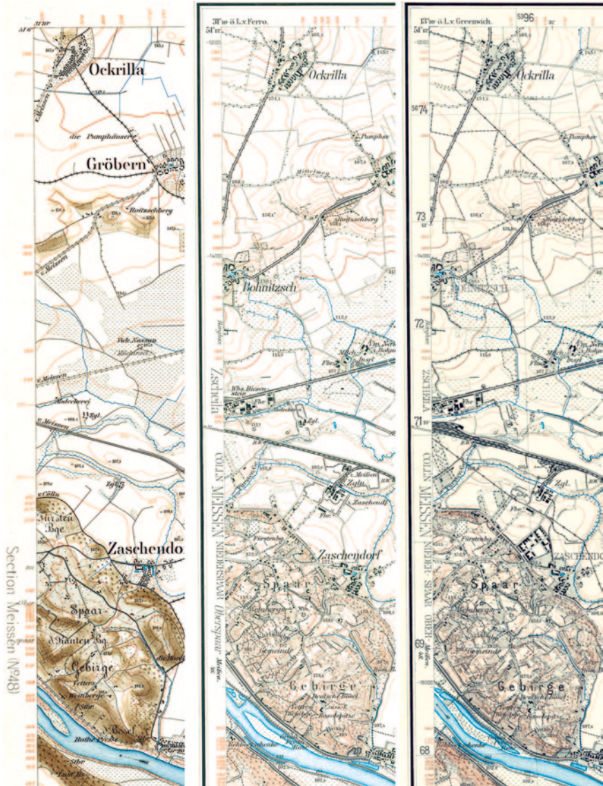
Fig. 11 Map comparison with regard to sheet lines, prime meridian and coordinates, as well as graphic representation. Left Äquidistantenkarte, sheet 49, 1882. Middle Messtischblatt, sheet 49, 1911. Right Messtischblatt, sheet 49, 1922. All sections: original scale 1:25,000—reduced (all: Sächsische Landesbibliothek—Staats- und Universitätsbibliothek Dresden, SLUB/KS 15307; SLUB/KS 15316; SLUB/KS 15325)
