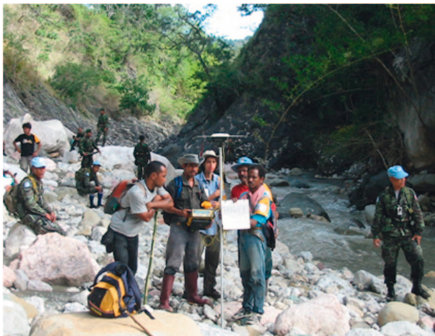
Fig. 4 The joint survey team conducted a GPS measurement of a delineation point in the middle of a stream
