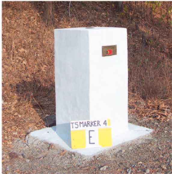
Fig. 5 An example of the border marker facing the East view with a plate showing the Timor-Leste flag (Courtesy of PPBW, BAKOSURTANAL, 2005)
