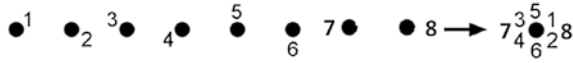
Fig. 2 Hierarchy of optimal label positions for a point object, from 1 (best) to 8 (worst)
