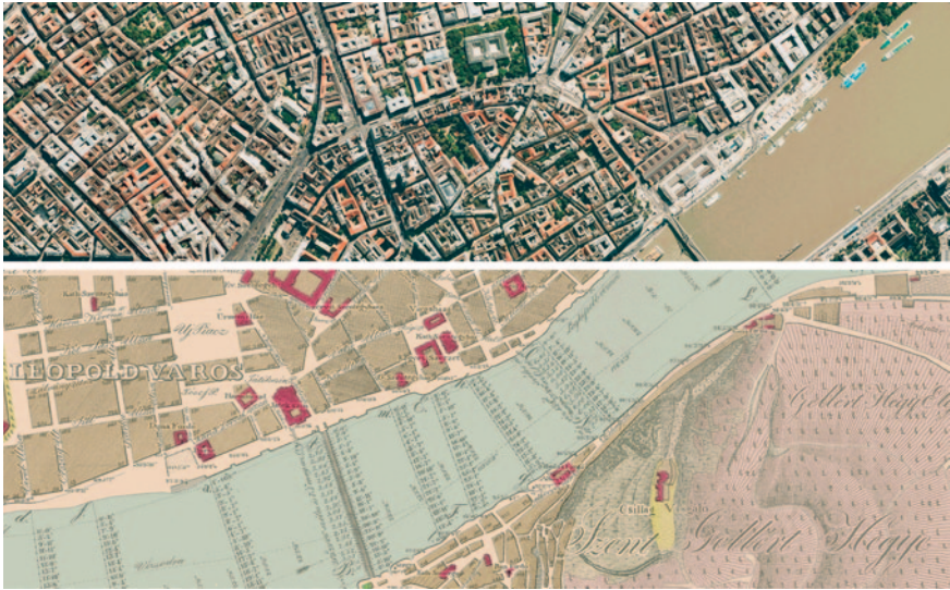
Fig. 7 Spatio-temporal comparison of the 1833 map and the 2012 satellite image. The detail with the city of Budapest demonstrates changes as well as the accuracy of the georeferencing
