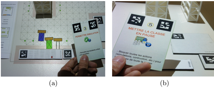
Fig. 3. (a) The “Allow Simulation” TinkerKey to allow/block simulation for a group, (b) The “Pause Class” TinkerKey to pause the whole class
