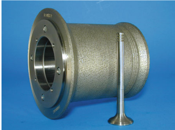
Fig. 13.40 Profile roll with workpiece (works photo Dr. Kaiser GmbH, Celle)
