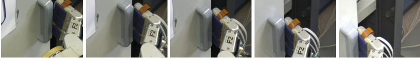
Fig. 7.10 A sequence showing the vision-tactile-force alignment process during task execution, starting from a coarse initial position
