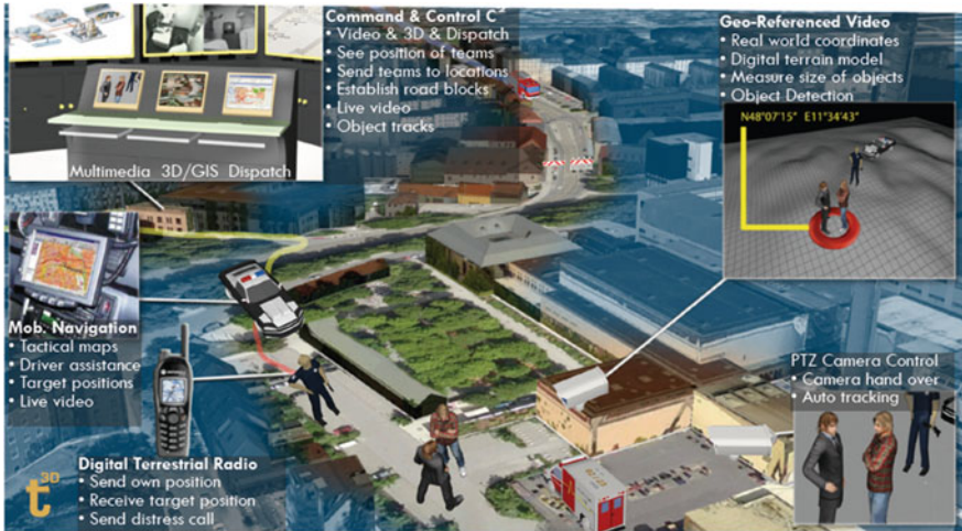
Fig. 5 Terra 3D incident management platform: geo-referenced video calibration procedure
