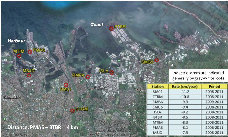
Fig. 6 Location of several GPS stations and their estimated land subsidence rates in Semarang; after Abidin et al. [9]. Subsidence rates are based on four GPS surveys since 2008 up to 2011
