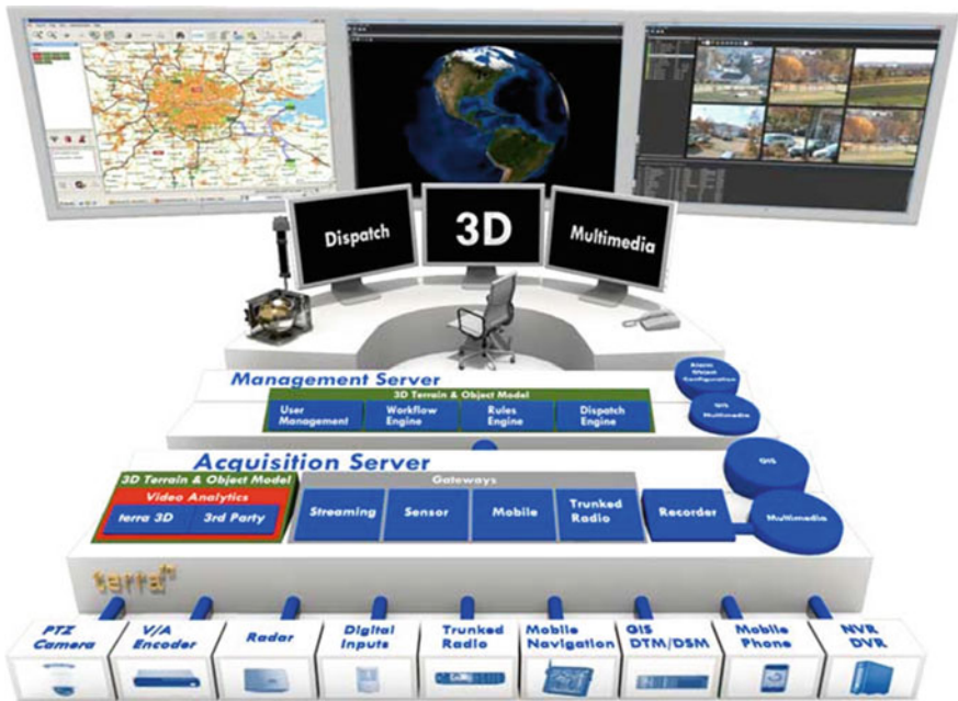
Fig. 6 Terra 3D incident management platform: multi-layer architecture
