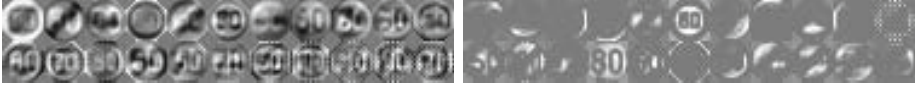
Fig. 1. Visualised PCA and NMF basis vectors with size of 17 \times 17 pixels. Left: PCA basis vectors, known as eigenfaces in face recognition applications; black pixels are negative values, white pixels are positive values. Right: NMF basis vectors; grey pixels are zero values, white pixels are positive values.
