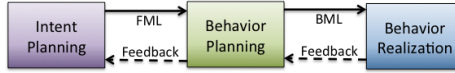
Fig. 1. The three stages of behavior generation in the SAIBA framework and the two mediating languages FML and BML. [9, 6]
