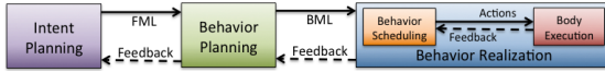
Fig. 2. Our subdivision of SAIBA’s Behavior Realization layer into the Behavior Scheduling and Body Execution sub-layers
