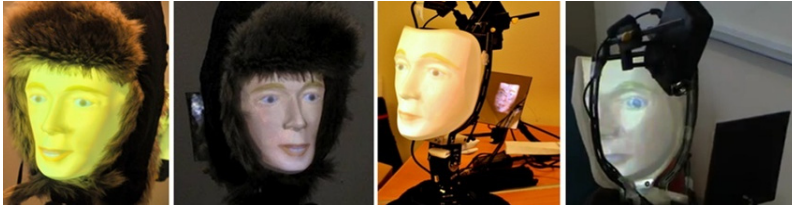
Fig. 1. photos of how Furhat looks like from the inside and outside
