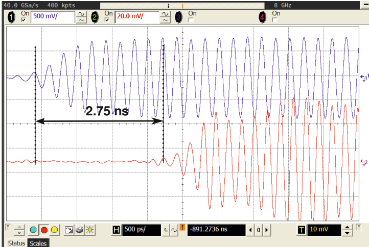
Fig. 9. Prover path delay: The total delay incurred due to mixing, filtering and channel activation switch is estimated to be 2.75ns
