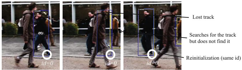
Fig. 5. Detailed reinitialization process of a track after an occlusion with an undetected person
