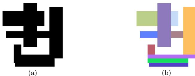
**Fig. 5.** (a) The binary convolution kernel used in the experiment. (b) Its 10 blocks of GBD decomposition.
