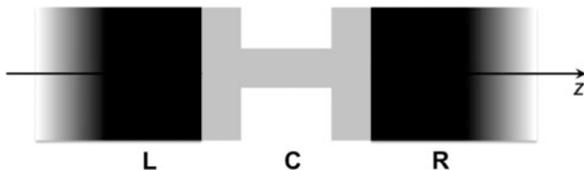
Fig. 1 Schematic picture of the division of the system into a central contact ( C ) and left ( L ) and right ( R ) electrode regions. The z axis corresponds to the transport direction
