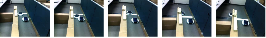
Fig. 3. An example of a robot giving way. After bumping each other, both robots move back and one exits the girdle to make room.
