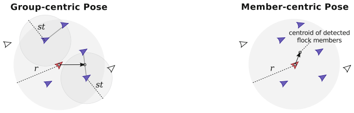
(a) The sensing flock member chooses the largest subset of the detected flock members and moves towards that group's average pose.
