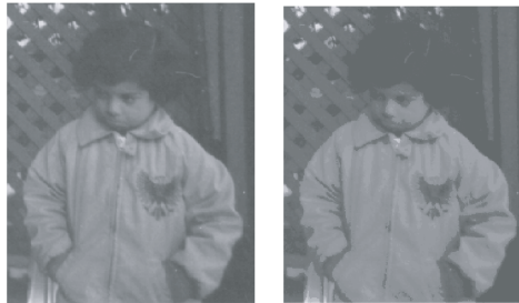
Fig. 12 Second Test Case Mean Shift Algorithm. The original picture can be seen at the left, and the one with mean shift algorithm on the right.
