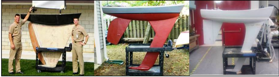
Fig. 4 SOA’s original(left) and modified (center) keel shapes with W2H
