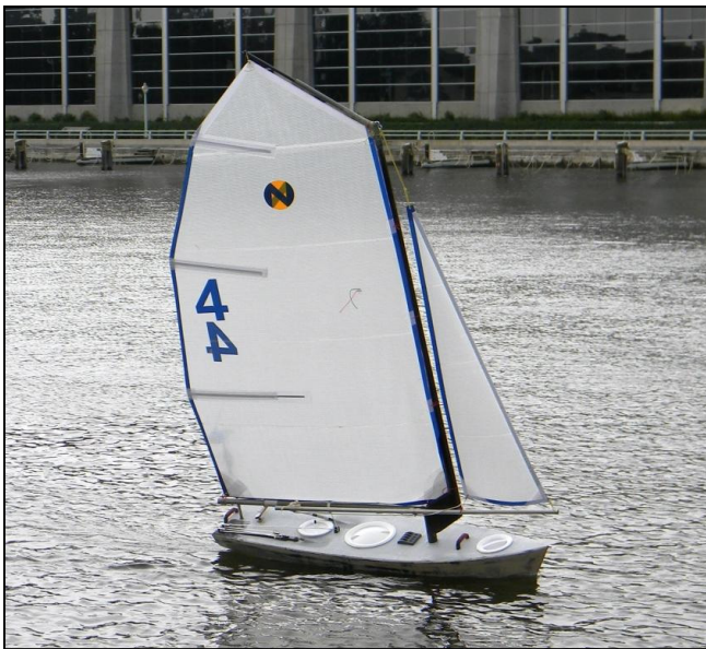
Fig. 7 SOA sailing with a balanced Balestron sloop rig in light air. The larger rig consists of boom and gaff extensions and the addition of a jib that rotates with the mast.
