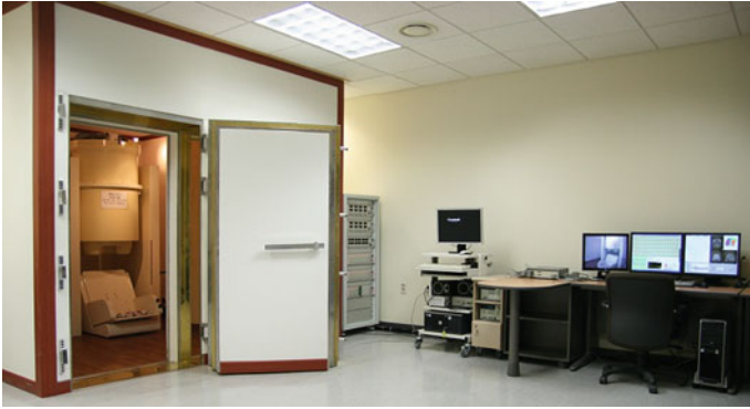
Fig. 11 A picture of a MEG system installed in a hospital. Helmet-shaped liquid He dewar mounted on a nonmagnetic gantry and inside a magnetically shielded room (MSR). Stimulation devices, acquisition, and analysis devices are outside MSR
