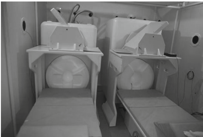
Fig. 2 Appearance of the child MEG system (left) and the conventional MEG system (right)
