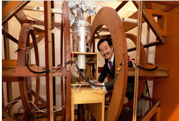
Fig. 29 A micro-Tesla NMR/MRI system. The measurement is conducted under a micro-Tesla magnetic field. All the detection and coil systems are placed in a magnetically shielded room
