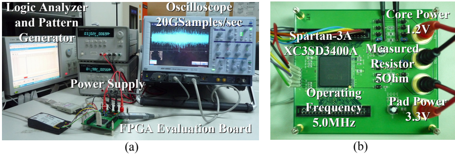
Fig. 7. (a) Environment of power measurement. (b) Current running through the DF-ECC processor recorded by measuring the voltage drop via a resistor in series with the board power pin and FPGA power pin.
