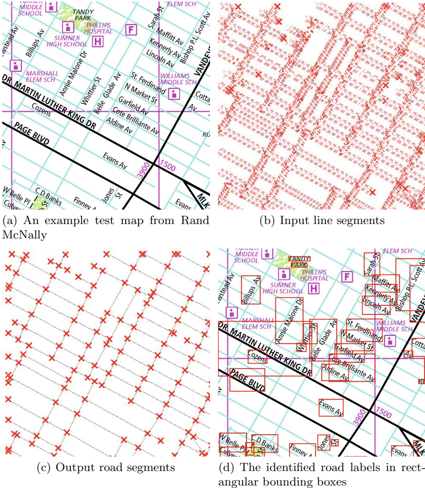
Fig. 6. Example inputs and intermediate results for grouping road segments and determining the locations of road labels
