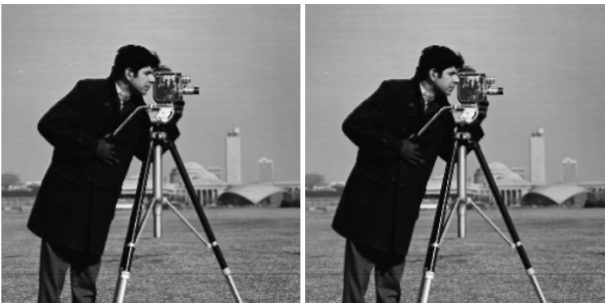
Fig. 3. Left: without histogram restore, PSNR = 29dB. Right: with histogram restore, PSNR = 30dB.
