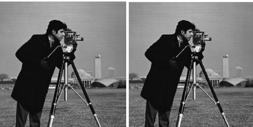
Fig. 6. Left: JPEG, CR=0.25, PSNR=39dB; right: JPEG, CR=0.43, PSNR=46dB
