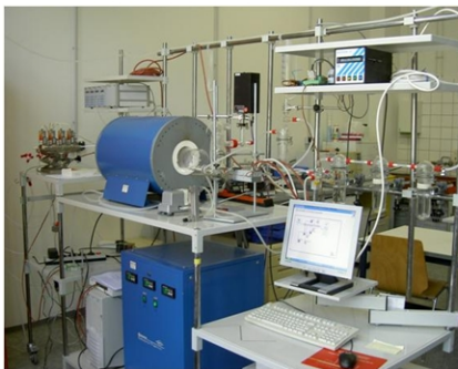
Fig. 4 Furnace with quartz glass reactor for thermo-chemical treatment
