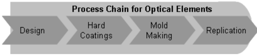
Fig. 4 Typical Process Chain for Optical Elements
