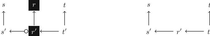
Fig. 2. Effect of routine Backtrack in the presence of candidate vertices s, r and t , each with a single primed predecessor vertex in their partition; the partition of candidate vertex r we wish to remove is highlighted, and the single conflicting edge is marked with “o” (left). After the call, the partition of r is removed and its former predecessor vertex r' is associated with s (right).
