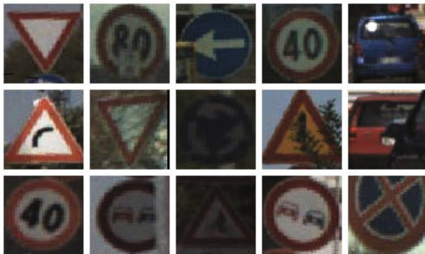
Fig. 3. Some results of the system. The first three columns show signs that have been correctly detected and classified, the fourth shows misclassified signs, while the last one shows wrong detections. Our method is robust against differences in light conditions and partial occlusions.
