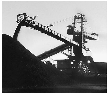
Fig. 1. A railed coal stacker building a heap
