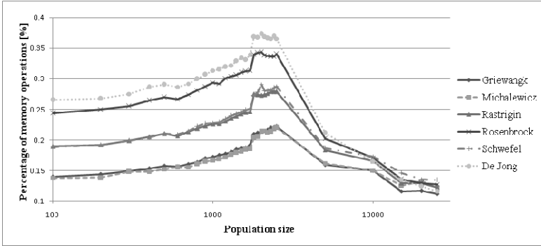
Fig. 3. Share of data transfer time on algorithms runtime with relation to population size
