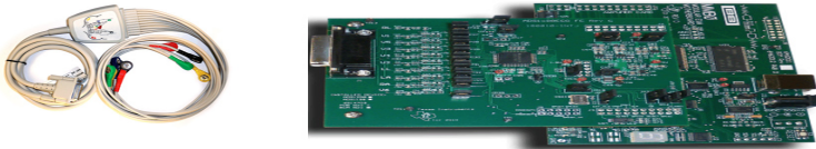
Fig. 9. Analog-to-digital acquisition board and cable connector to capture EEG signal
