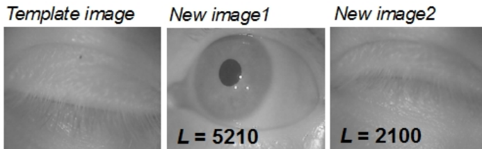
Fig. 2. The example of L2norm values by comparing template and new image
