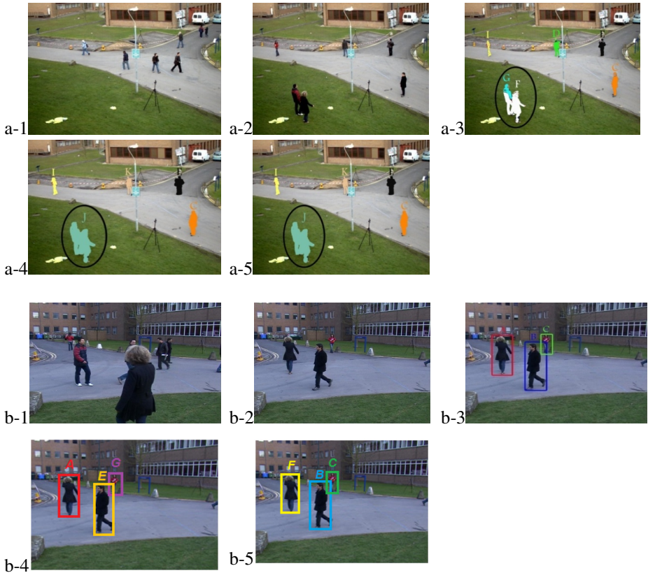
Fig. 5. some results of tracking process: a-1 is frame number 245 and a-2 is frame number 469. a-3 shows the tracking results using proposed method that can detect F & G objects correctly (with some pixel detection errors). Note that F & G objects are present in the frame 245(a-1) but they are so far and they come closer in the frame 469. a-4 shows the tracking result using classic GA that lost the F & G object from frame 245 to 469 and get them a new incorrect index. a-5 is the result of PF method that made a mistake similar to classic GA. Our proposed method can detect object A from the frame number 260 (b-1) to frame number 452 (b-2). Note that object A is going far from camera and its size is variable. The PF method lost the object A (b-5) but the Classic GA track this objects although it is lost some others.
