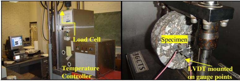
Fig. 1. Creep Compliance Setup
