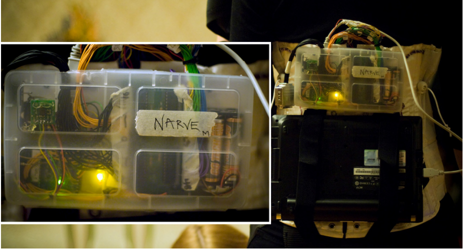
Fig. 1. Controller box with DUSK board (64 actuators) for BlindTheatre Bodysuit
