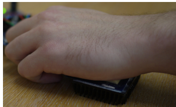
Fig. 2. Thenar placed on Peltiers
