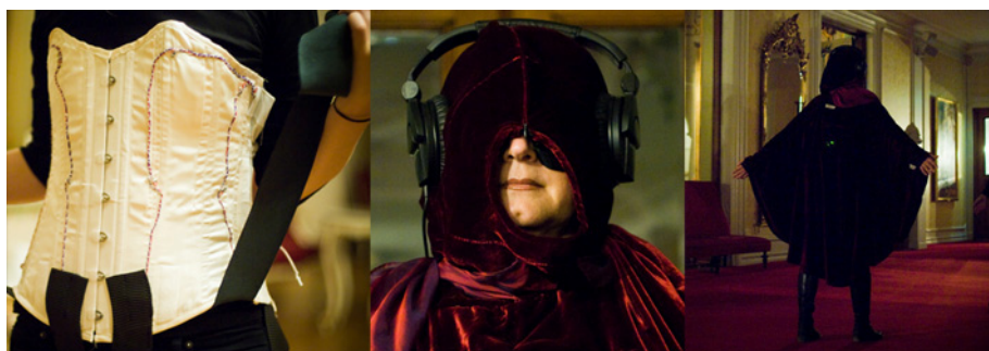
Fig. 2. The bodysuit for the Blind Theater. The haptic suit had two functional layers, one inner corsette and an outer, looser-fit cape.
