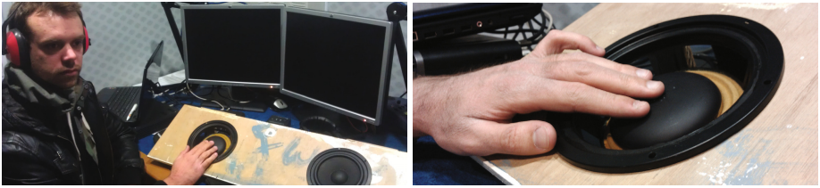
Fig. 1. (left) Haptic test stimuli protocol, including the use of noise-suppression headphones. (left driver) Cone removed and added dome for haptic stimuli, (right drive) unmodified for audio stimuli. (right) Hand of a participant, showing the wrist resting on the wooden board and the three mid-fingers placed on the plastic dome.
