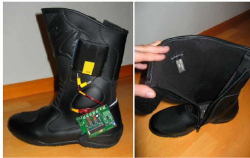
Fig. 5. Shoes providing tactile feedback for cyclists to support their training
