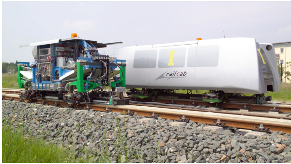
Fig. 5.12 Photograph of the RailCab test vehicle
