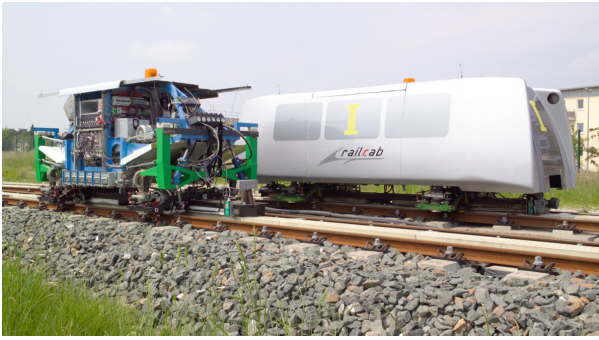
Fig. 5.12 Photograph of the RailCab test vehicle
