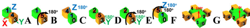
Fig. 3 (A)-(F) Examples of SuperBots with identical 3D shapes. In B, E and, F, the middle servo rotates 180° (G) Two isomorphic configurations with a module rotated around a symmetry line.
