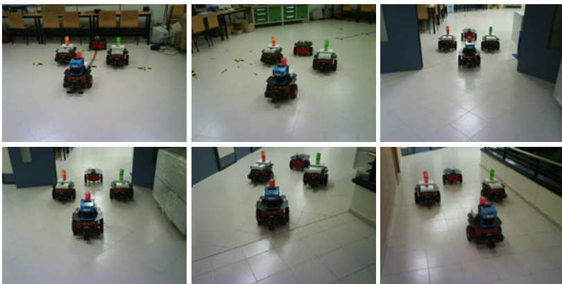
Fig. 8 Test with four-robot diamond formation using visual repositioning
