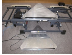
Fig. 2 Two specially designed force plates placed at the positions of the feet and hip of subjects
