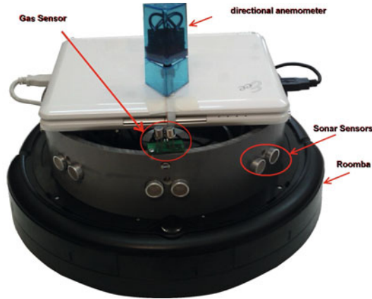
Fig. 8 iRobot Roomba robot equipped with a laptop, a sonar array, gas sensors, and 2D anemometer
