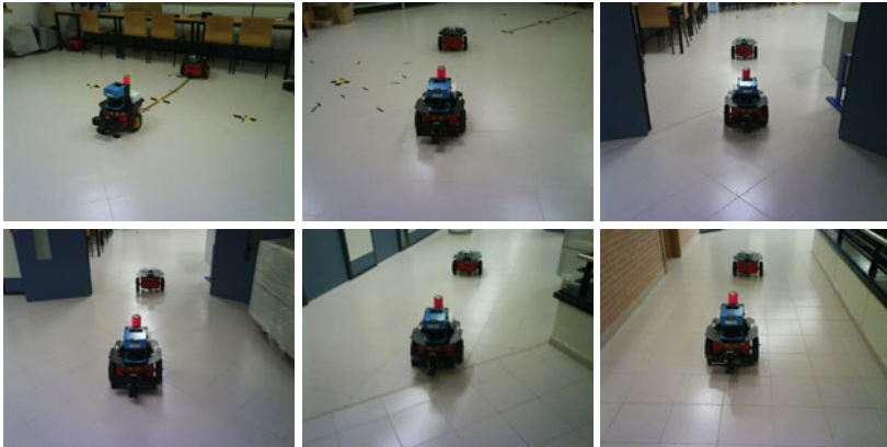
Fig. 7 Test with two-robot leader-following formation using visual repositioning
