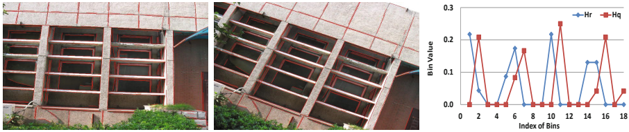
Fig. 1. Illustration of line direction histograms. The first two images show the reference and query images with detected lines and the plot shows their direction histograms. The resolution of each bin is 20 degrees, so there are 18 bins for each histogram.
