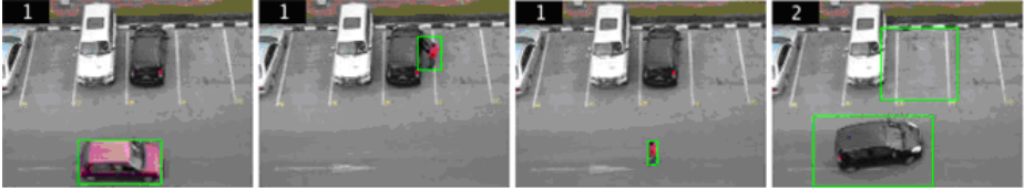
Fig. 4. Object tracking result of the test video. From left to right, car passed by the scene, people walked by the scene, people picked up a car, and car moved out of the parking space.
