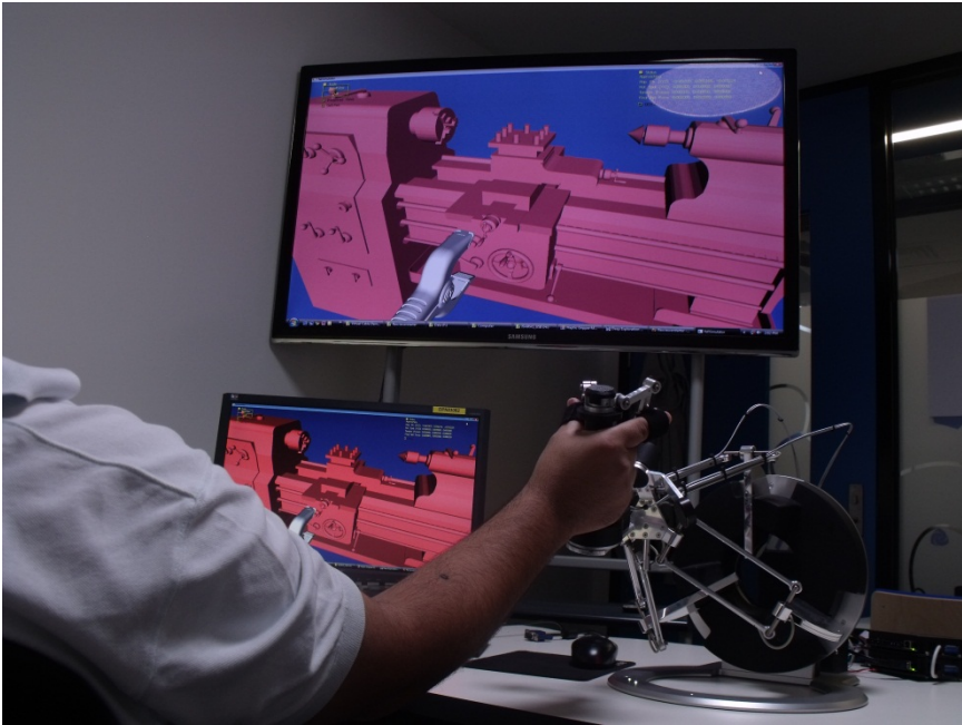
Fig. 11. Function-based collision detection and force rendering of haptic assembly scenario
