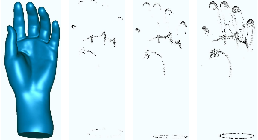
(b) Hand model (39325points) with \alpha from left to right assigned to 4.5 (372points), 3.5 (880points) and 2.5 (2228points), respectively.
