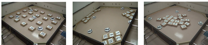
Fig. 1. (left) initial configuration, (center) an example final configuration using the basic strategy, and (right) an example final configuration using the mixed strategy (2 Twisters and 3 Diggers). Video clips are available at http://students.cse.tamu.edu/jnk3355/experiments.html
