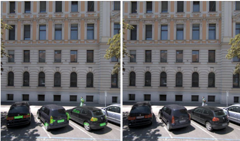
Fig. 11 Privacy detection by marking areas assumed to contain private information, and subsequently making these areas unintelligible (Kröpfel et al. 2012)
