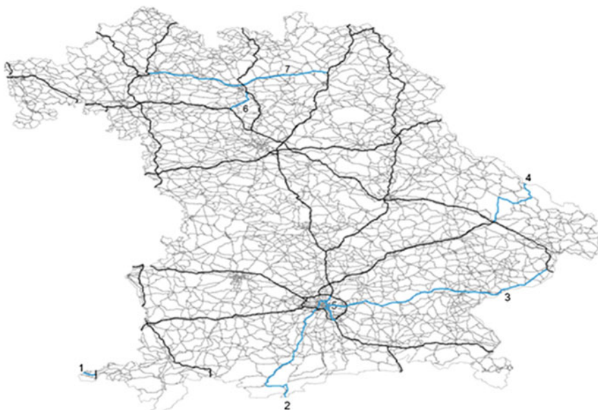
Fig. 11 Decisive paths (in blue ) detected by the OPCV algorithm in Bavaria state
