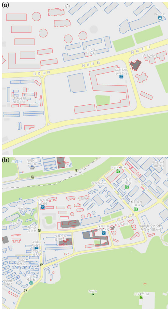
Fig. 6 Overlay of electronic maps (updated objects with red boundaries, invariable objects with blue boundaries, the inconsistencies of overlay filling with black ). a Overlay of 1:2000 electronic maps. b Overlay of 1:5000 electronic maps
