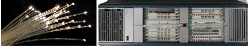
Fig. 3 Fiber bundle ( left ) and aso-called “core router” ( right ), example of a current contemporary CISCO Internet-device (from en.wikipedia.org/wiki/Core_router )
