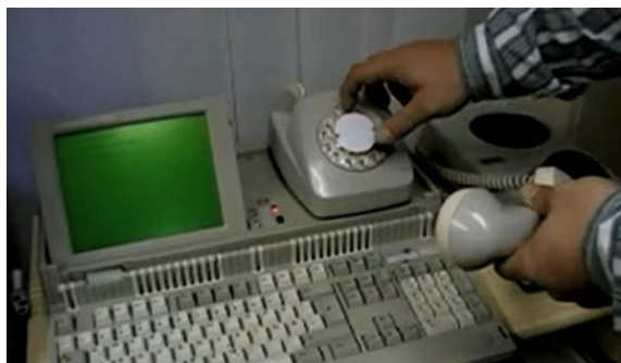
Fig. 2 Acoustic coupling of two computers via a telephone line—
