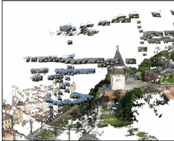
Fig. 12 MAV-based imaging into an irregular assembly of aerial images, and extraction of a dense point cloud of the clock tower in Graz (from http://www.youtube.com/watch?v=vYXhVG7VMY0 )
