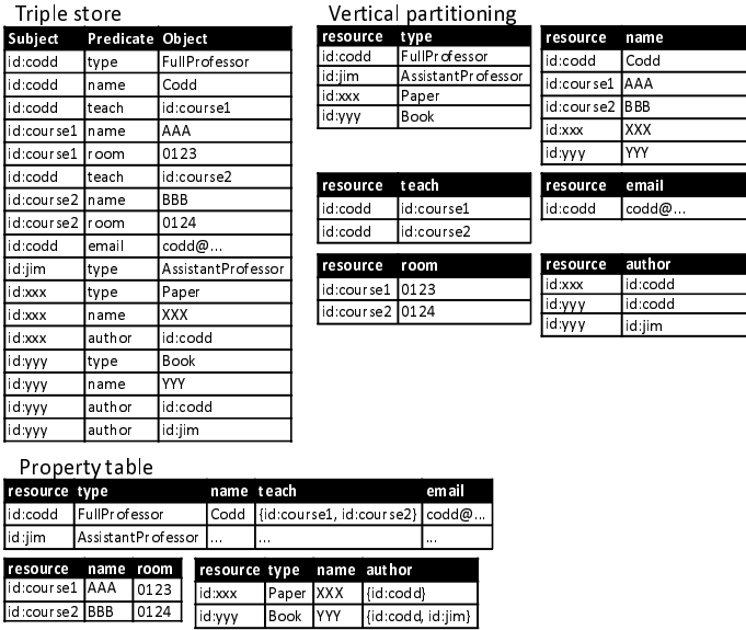
Fig. 1. RDF storage schemes; (a) Triple store (b) Vertical partitioning (c) Property tables
