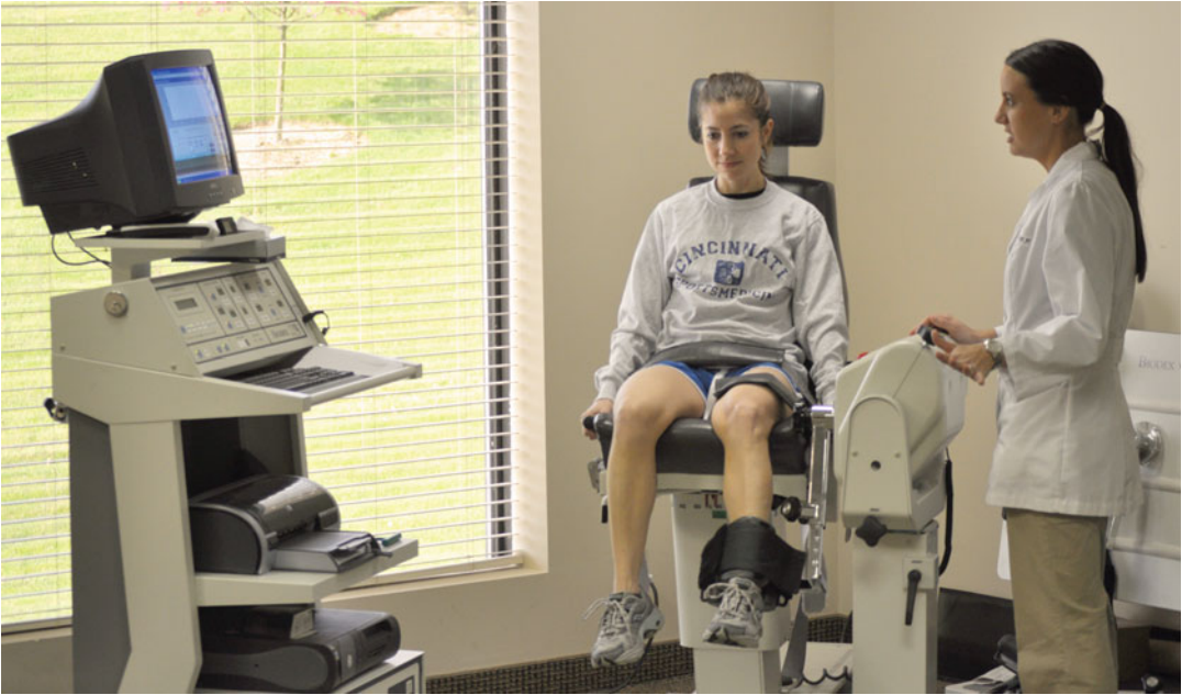
Fig. 18.4 Isokinetic knee flexion-extension strength test on Biodex isokinetic dynamometer (Biodex Corporation, Shirley, NY)
