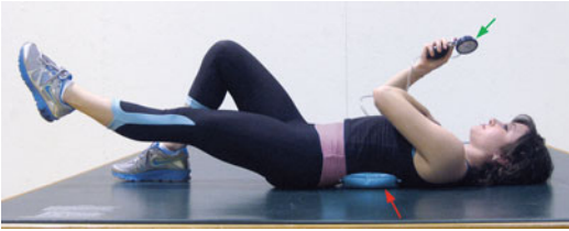
Fig. 9.2 Clinical test of supine trunk control. An air bladder is placed under the lumbar curve ( red arrow ) and inflated to a known pressure as indicated by a pressure gauge ( green arrow ). Subjects perform arm or leg lifts while attempting to maintain the curve, and increased or decreased air pressure in the bladder indicates a lack of control of spine movement. This apparatus can also be used as biofeedback during training exercises where the goal is to minimize changes in pressure
