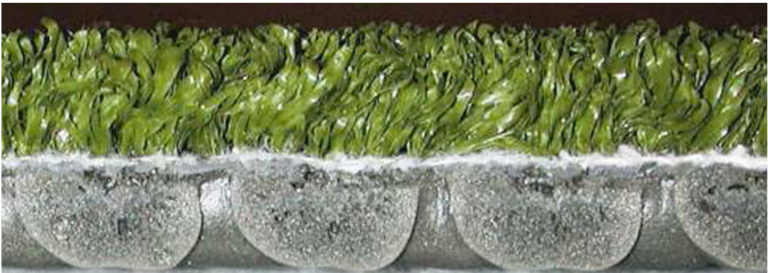
Fig. 4.6 First generation artificial turf. 10–12-mm fiber length, integral shock pad, nylon, unfilled, hard, and abrasive. Developed in the 1960s [34] (Reprinted by permission of Loughborough University)
