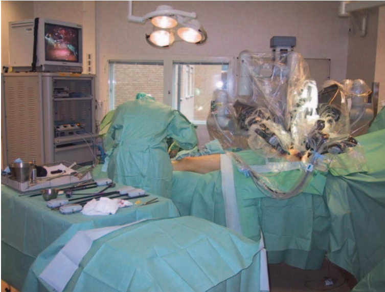
Fig. 2.4 The robotic arms occupy the space around the patient where the head surgeon and surgical assistants would normally stand (see Fig. 2.2). In robotic mitral valve surgery, the head surgeon controls the robot remotely through a console. Although assisting staff members are more spread out in the operating theatre, they are still required to be in close proximity to the patient and the robotic arms. © K. Wasen
