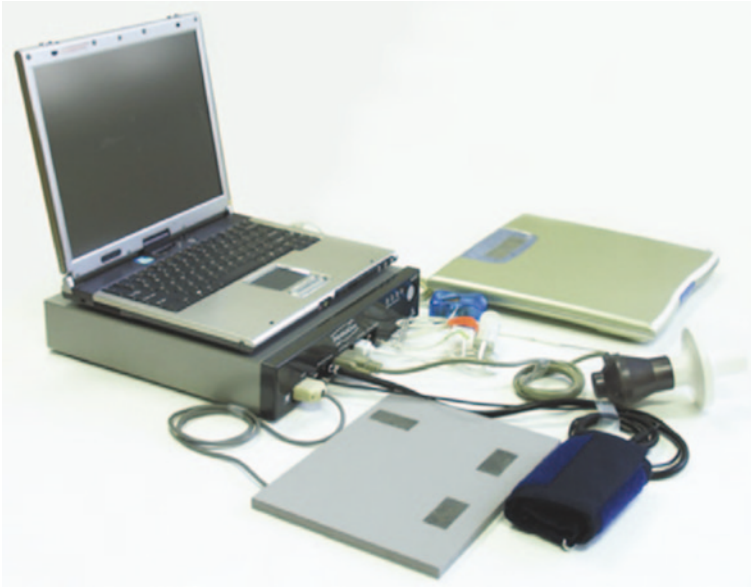
Fig. 4.2 The home telecare patient unit as demonstrated in the focus groups, showing the computer screen with clinical measurement unit underneath and the various peripherals used for physiological recording. These include a wireless weight scale, single lead electrocardiogram, blood pressure cuff, spirometer, and pulse oximeter
