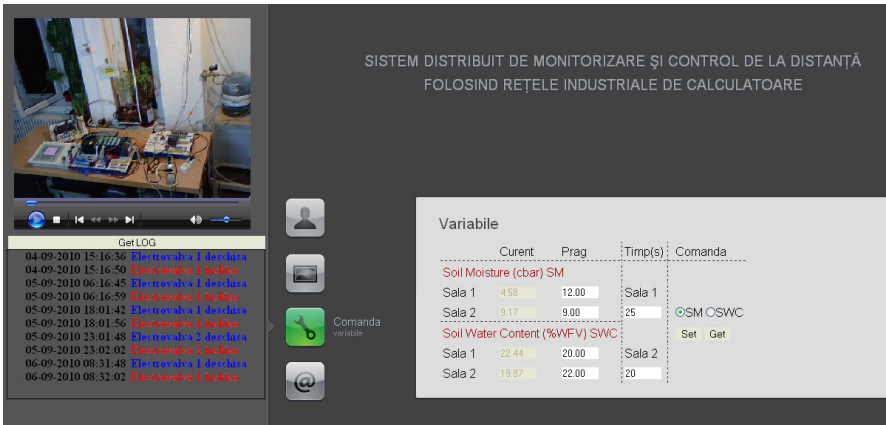
Fig. 7. The web interface for remote process control
