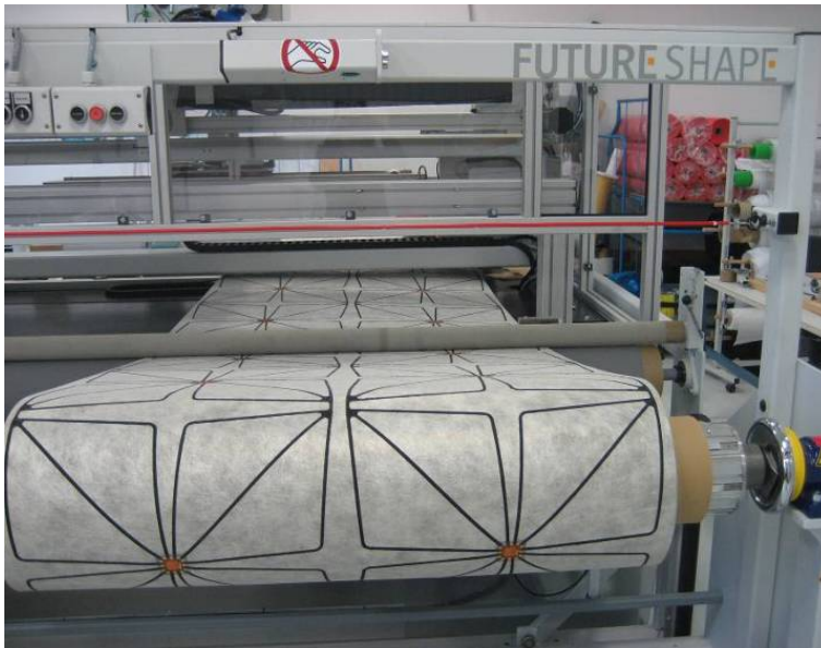
Fig. 8. Roll-to-roll production of the SensFloor underlay. In this picture the integration of the radio modules (four per square meter) into the sensor underlay is done.
