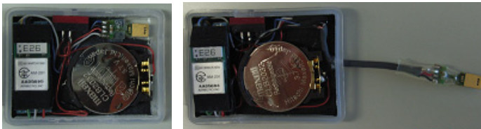
Fig. 4. First version of thermo-hygrometer (left) and skin temperature sensor (right). (The cases are opened.)
