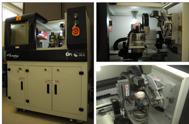
Fig. 1 Micro X-ray CT equipment of KICT (a) view of micro CT scanner (left), (b) arrangement of three major parts (source, manipulator and detector from right hand side, respectively in upper right figure), (c) zoomed manipulator & detector (lower right)
