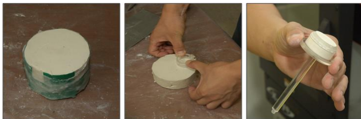
Fig. 2 Sampling process: (a) cutting (b) sampling (c) ready for CT scanning
