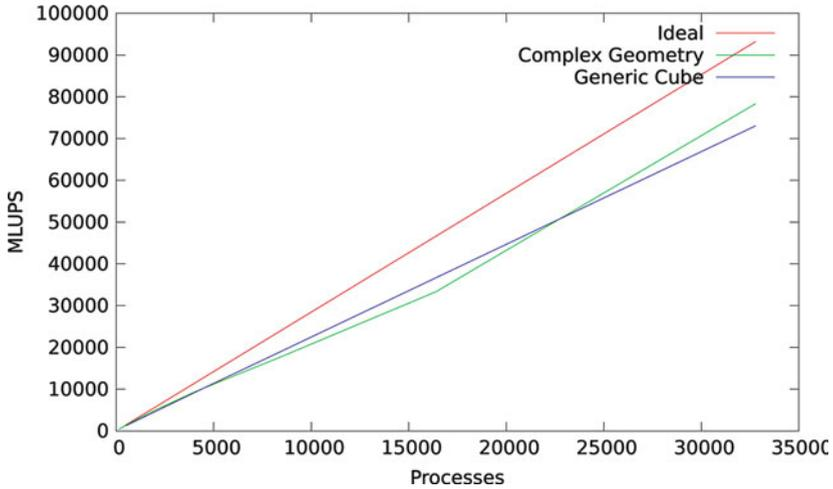
Fig. 1 Speed up comparison on Hermit between domains with geometry and without
