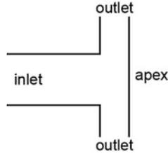
**Fig. 2** Initial flow geometry, inlet, outlets and the apex are indicated
