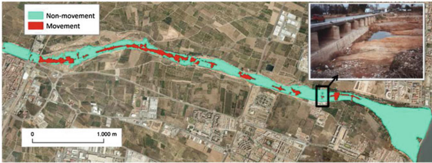
Fig. 1 Mobilized and non-mobilized areas in the Palancia river basin as predicted by the hydraulic-sedimentological analysis performed in the studied reach. The detailed view shows the effects of sediment scour downstream the Canet bridge
