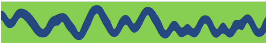
Fig. 1 Folded feldspathic vein (blue) embedded in quartzite (green). The initial thickness of the feldspathic vein is 2 m. The sample was buried at a depth of 10 km. The lateral dimension of the deformed sample is 500 m
