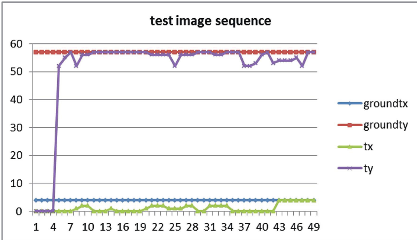
Fig. 4 The results of aligning IR and TV images, algorithm used: Canny simplified, in range \pm 64 pixels with smoothing filter; tx, ty - calculated values of translation in directions X and Y; groundtx, groundty - reference values of translation
