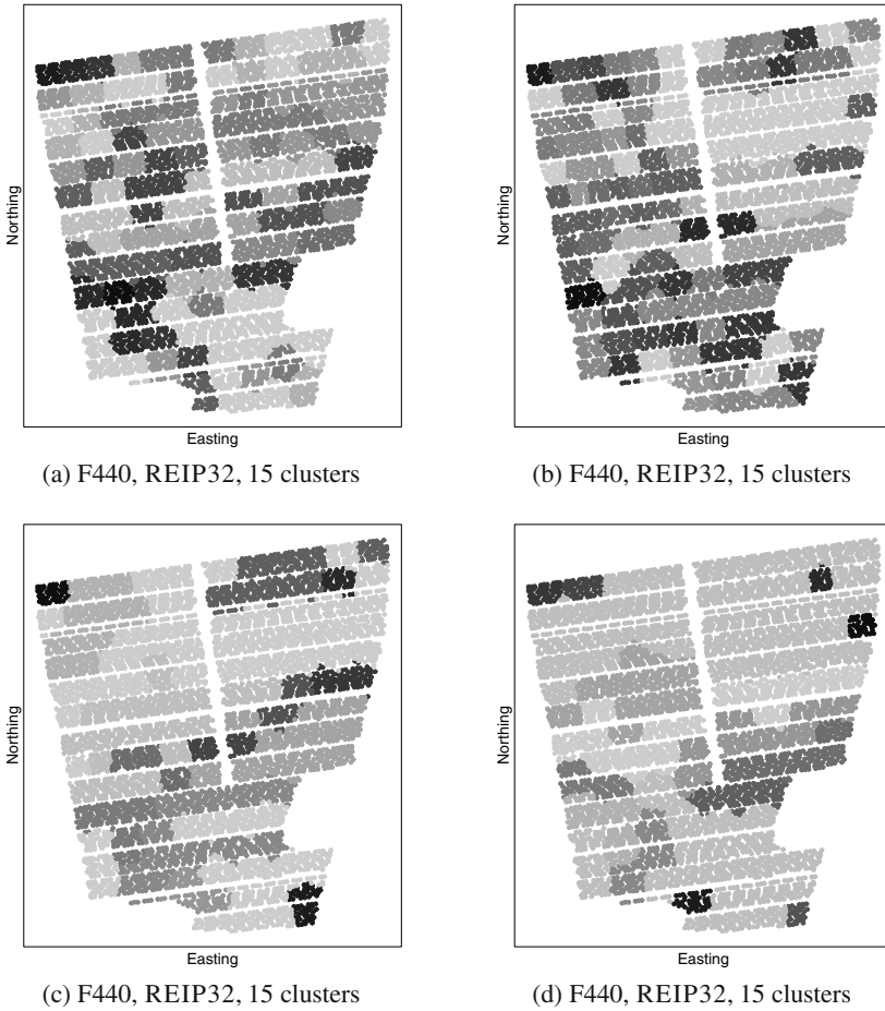
Fig. 3 HACC-SPATIAL on F440, 120 initial clusters, using the REIP32 variable and demonstrating the effect of different spatial contiguity settings. While (a) shows spatially rather scattered clusters, the change in the designed contiguity ratio threshold varies the spatial contiguity of the clusters until spatial contiguity is strictly enforced in Figure (d).
